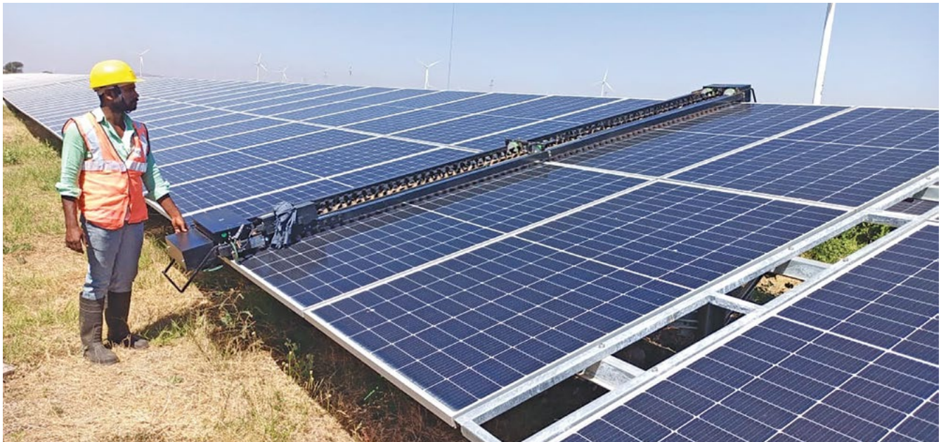
Robotic cleaning at one of the solar power plants financed by NIIF IFL, owned and operated by the Radiance group
